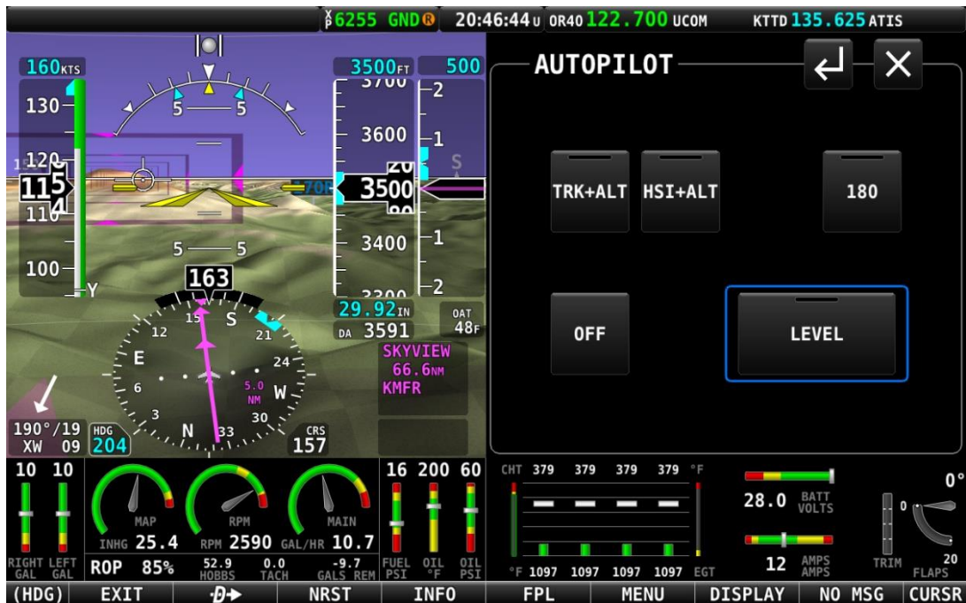
Figure 214 – AUTOPILOT Control page – Simplified Control Scheme
