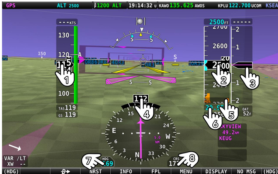
Figure 29 – Touchable on-screen regions that change Knob BUG Function; See Below for Legend
