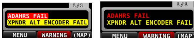
Figure 245 – Unacknowledged (left) and Acknowledged (right) Alarms
