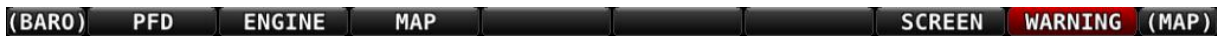
Figure 243 – Message Notification Area above button 8 (2nd from right), showing a Warning Notification
