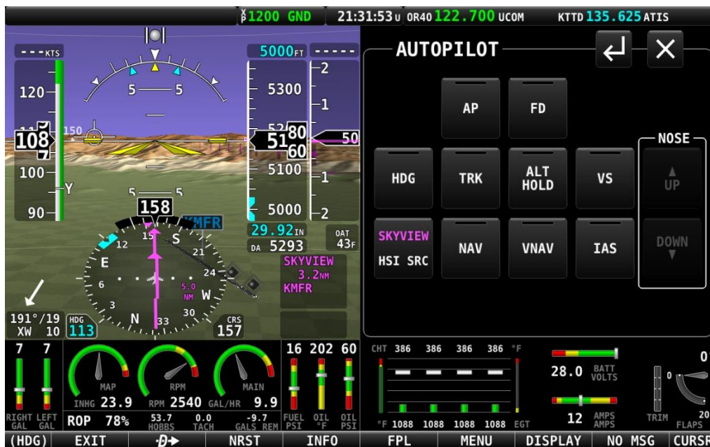
Figure 223 – AUTOPILOT Control page – Expert Control Scheme
