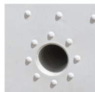
Heater Combustion Blower Intake
