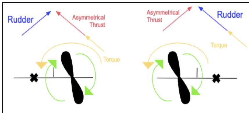
To counteract these P.A.S.T factors rudder pressure must be applied to the side of the operational engine. Hence the practice of "dead foot = dead engine".
