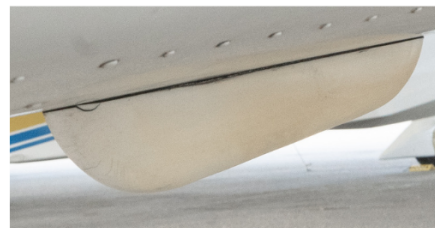
Marker Beacon Antenna
