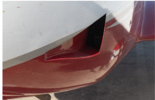
Induction Air Inlet
