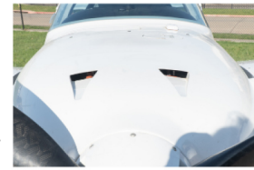
Air Cooling Inlet
