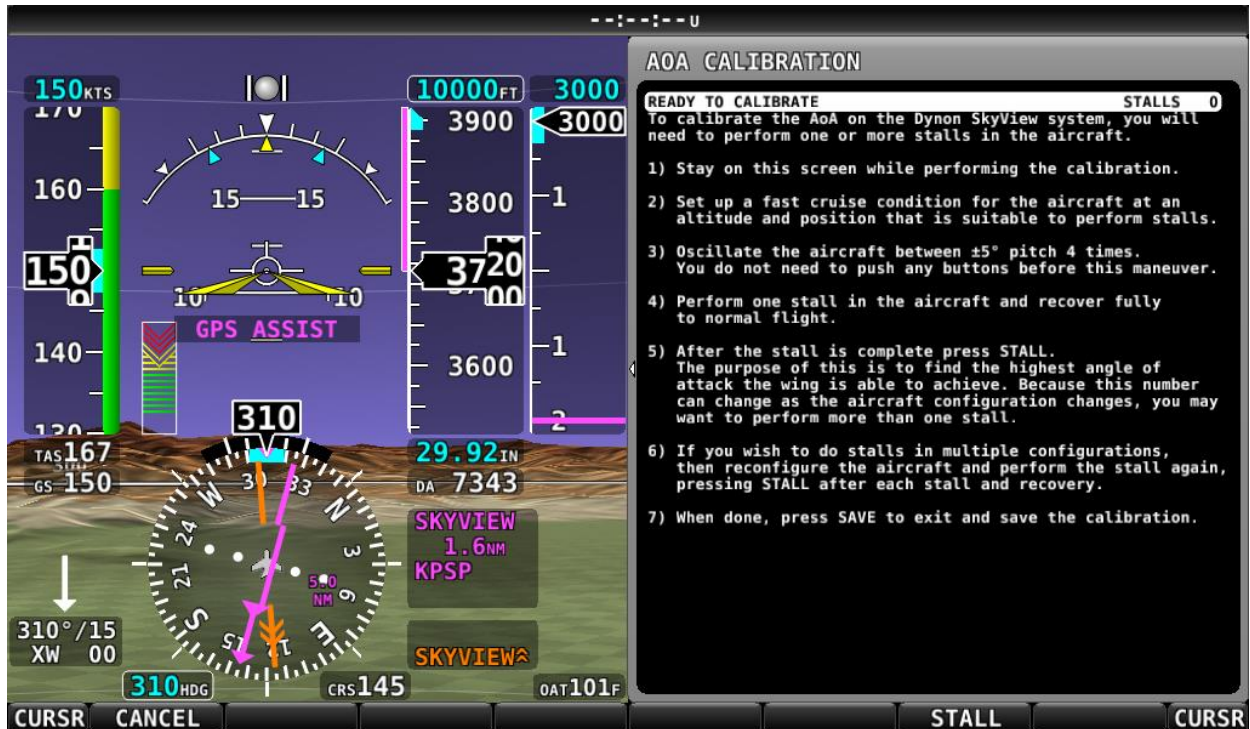
Figure 163 – AOA Calibration Explanation and Wizard
