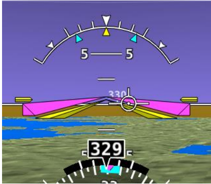
Figure 118 – Flight Director - Single Cue (Inverted-V)
