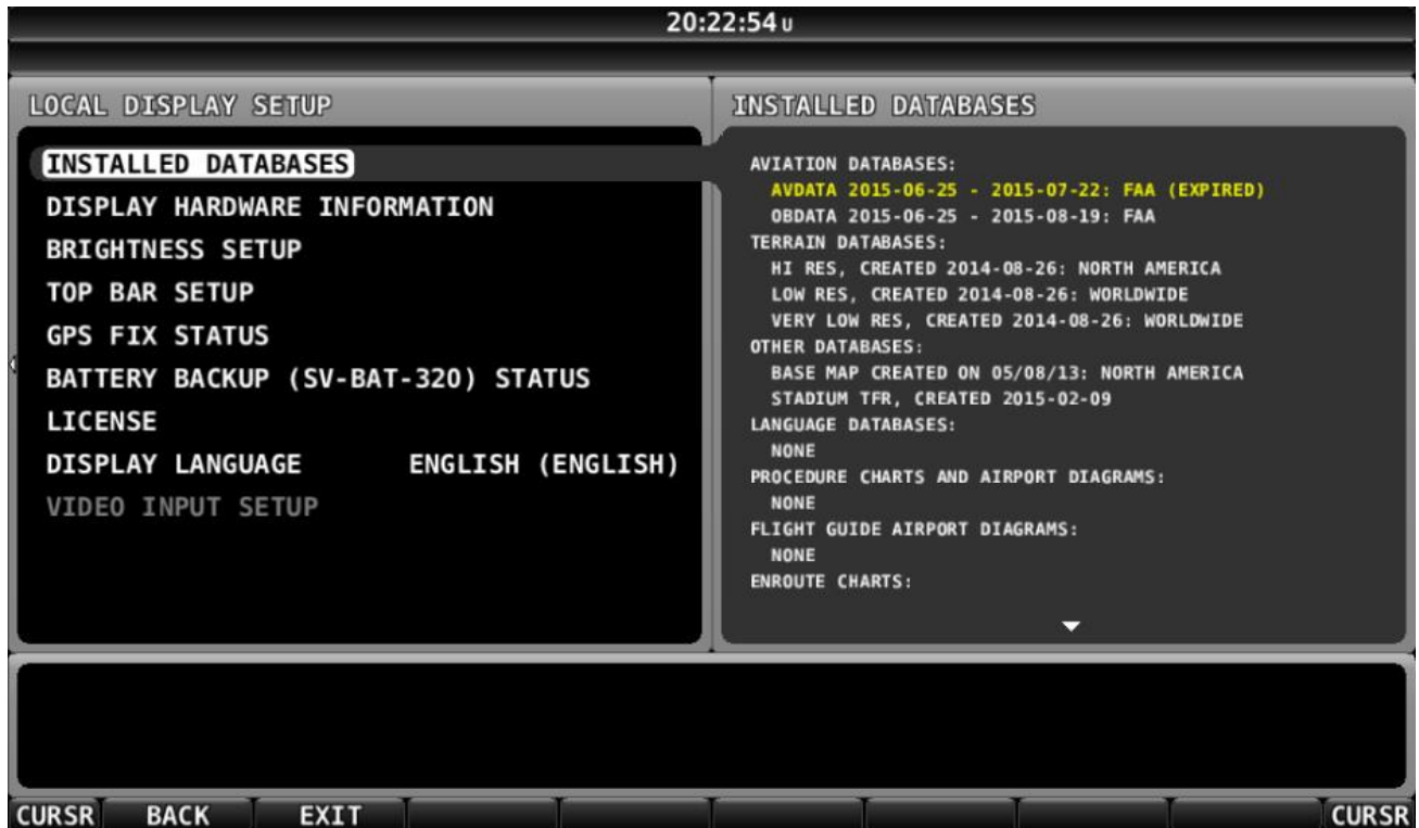
Figure 53 – SkyView INSTALLED DATABASES with Expired Database Shown in Yellow
